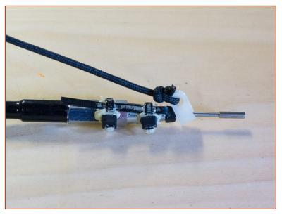
first in place. The friction tie must have a hole in the head the size of the whip.
