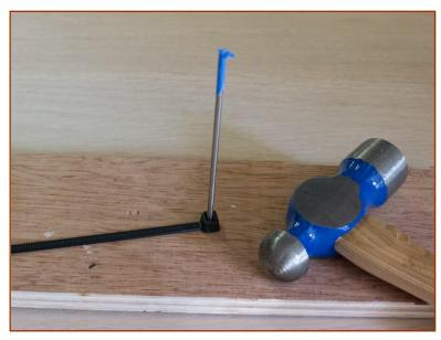
whips can be pushed into the coil segment of the antenna for storage. Not a bad solution that costs pennies.
