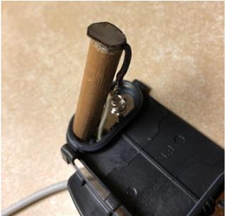
Now the contact will reach the exact distance into the battery pack to make a good contact, and you can drill a small hole in the battery compartment cover to bring the power wire in.
