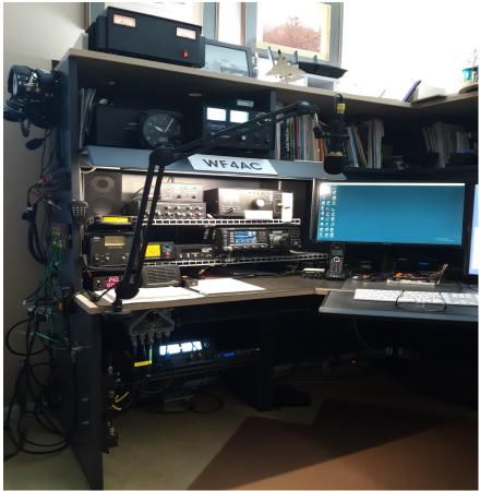
As an aside, I disconnect the ground strap, antenna leads and power plugs after each use. Just don't want any lightening to find its way into the shack. That includes the house ground via electrical plugs.
