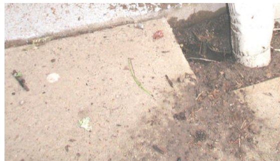
Figure 10b. Soil blown out around the top of a totally buried ground rod due to a lightning strike.
