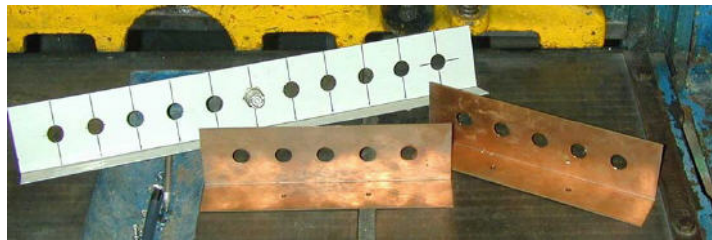
Figure 18. Shop made bulk head panels for single point grounding of incoming feed-lines. Picture from W8JI, www.w8ji.com .
