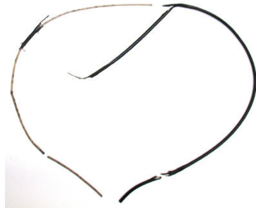
Figure 5b. Conductors sometimes do not survive a lightning strike either, as did not this section of RG-59. It was at the top of my 100 foot tower. The center conductor and shield were vaporized.
